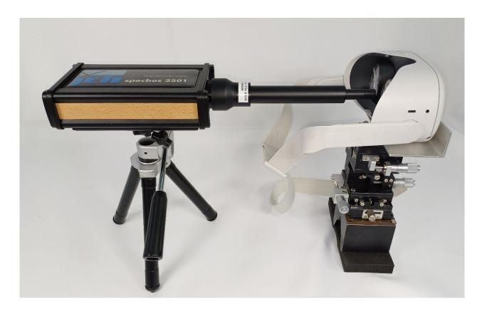
The ACC 089/3 add-on optics enables such a measurement in conjunction with specbos 2501.
