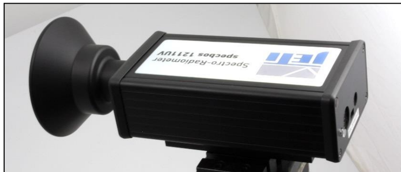
Fig. 4 Diffusor with 80° aperture (ACC 027)
