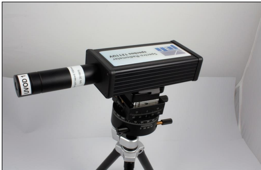
Fig. 8 Scheme of radiance based measurements (picture: specbos 1211-UV-2 with 100 mrad optics and additional OD1 filter)
