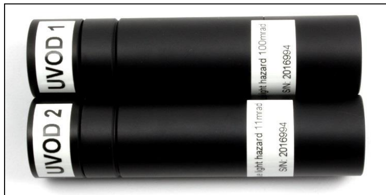
Fig. 5 Measuring optics with OD filters (in this case ACC 024/11 with external OD2.0 and ACC 024/100 with external OD1.0)
